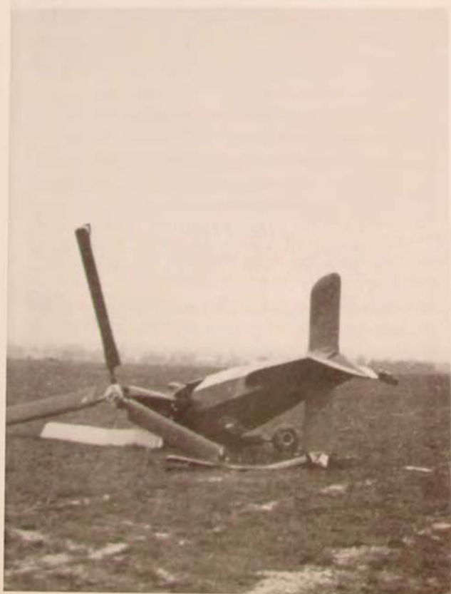
The autogyro (above) was powered by a free-spinning rotor and a conventional aircraft propeller. Unfortunately, it was so unstable that a good many of them ended up like the one shown at left.
