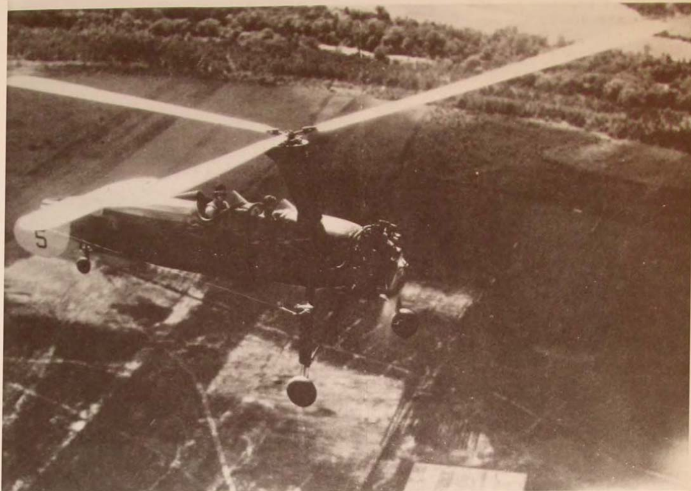
The autogyro (above) was powered by a free-spinning rotor and a conventional aircraft propeller. Unfortunately, it was so unstable that a good many of them ended up like the one shown at left.
